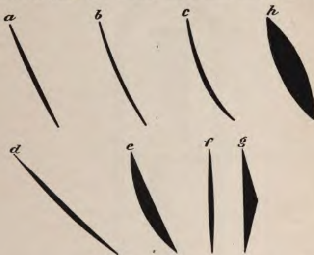
Fig. 14.—This drawing shows the ends of screw blades in which a is a plain screw; b , screw with increasing pitch; c , screw with compound increasing pitch; d , end of screw blade 45^\circ ; e , screw with very thick blade; f , blade with no pitch at all; g , blade which gave a thrust in the direction of the convex side, no matter in which direction it was revolved; h , screw said to have been used in the French Government experiments.
